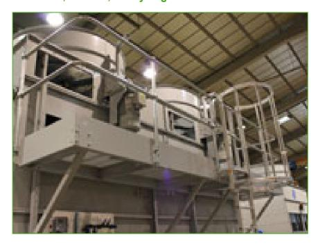
**Platforms, a ladder, safety cage and handrails** facilitate **easier and safer access** to the unit, making inspection and maintenance easier and conforming to European safety standards.
