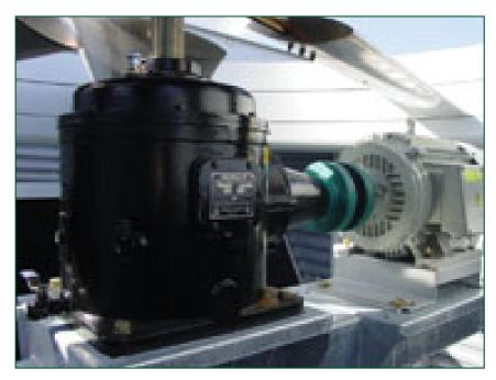
Factory-installed and aligned, the close coupled motor gear drive system is a good option for **certain industrial applications**.
