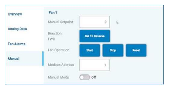
The Modbus address is only available for a specific fan, not when you have selected "All Fans". Set manual mode to "off", if normal operation needs to be resumed.
